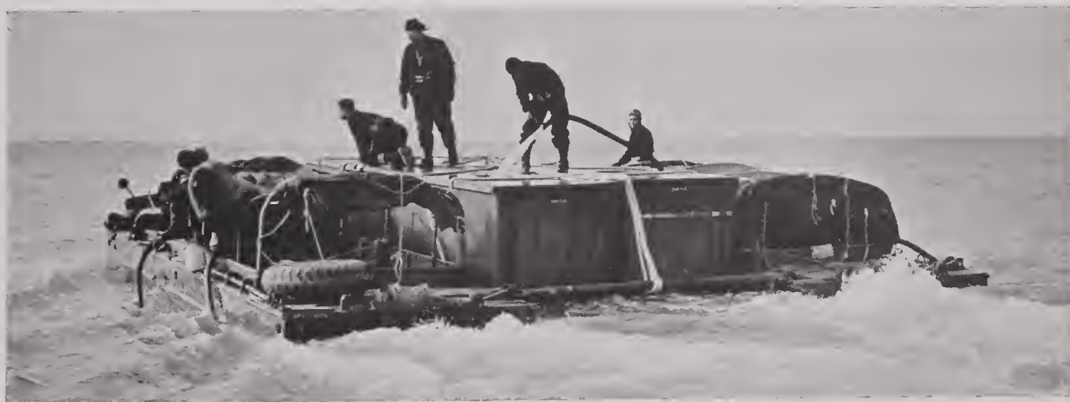
FIGURE 63. Rehearsal of wet ferry off Fort Story, Virginia, with boxes of water as test load.
